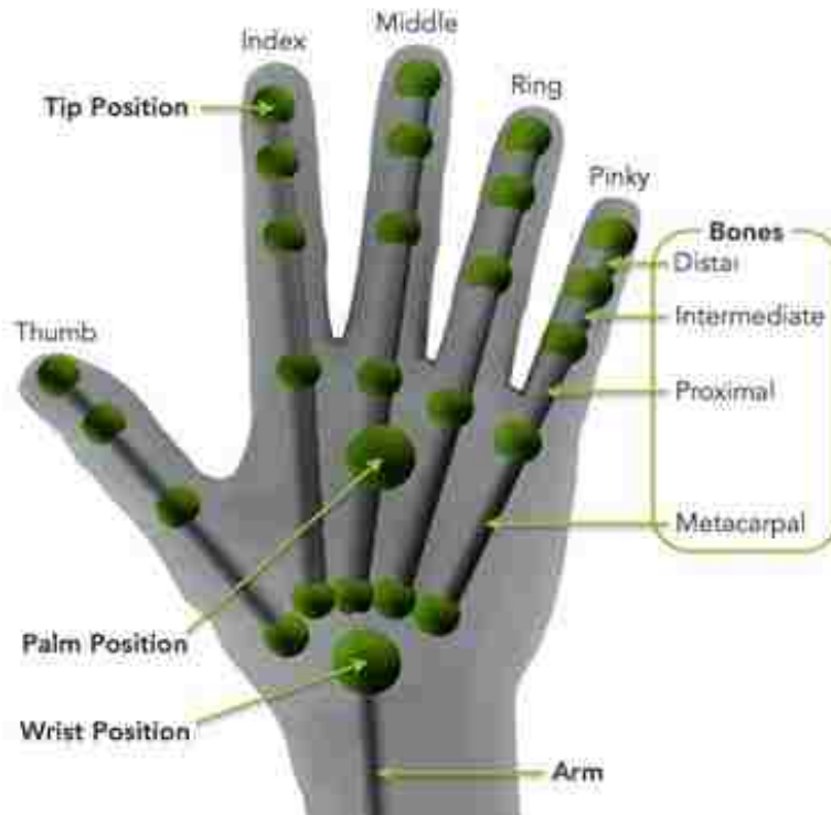
Figure 4.3.2. Example kinematic output from Leap Sensor API [39]. The Leap sensor provides direct access to individual joint positions (green spheres) as well as direction vectors (grey bars) of up to two hands at a time.
