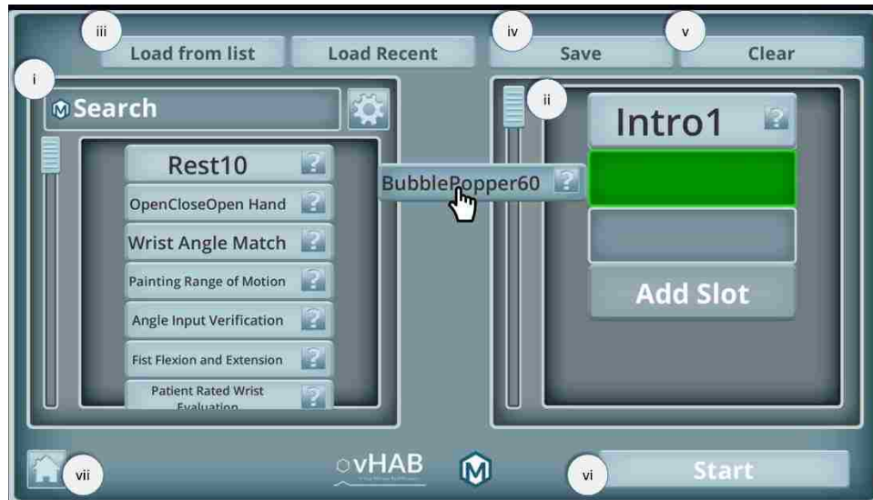
Figure 4.4.8. Assessment Select screen A6. This screen allows for the creation and loading of custom lists of assessment modules. Users can drag and drop modules from the left column listing all the modules to their custom list on the right. In this example, a user is dragging a module over to their custom list. The hand-cursor represents the user’s interaction point (either a mouse click or a screen touch). The green box shows where the module would be placed if the user let go of the BubblePopper60 module.
